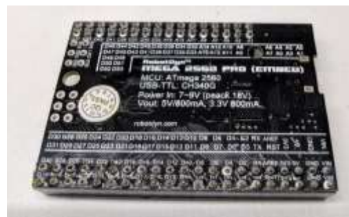
Figure Error! No text of specified style in document..3 Mega 2560 PRO Embed
