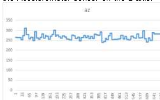
Figure 4.6 Accelerometer ADXL345 Sensor Response z axis.
